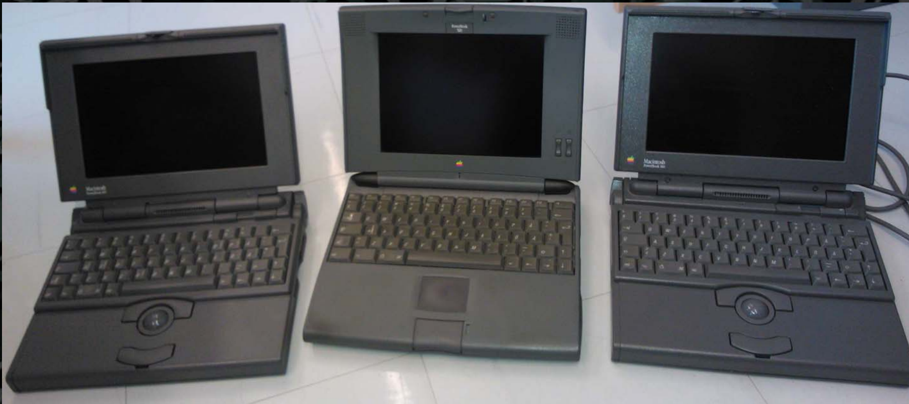
These computers work but have issues with connectors and system batteries (low voltage on battery, connectors break the current from time to time).
